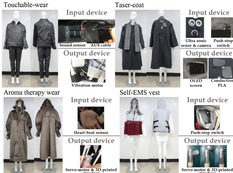
Fig. 16 The developed each prototype at the Stage of 'Build an Interactive Version'
